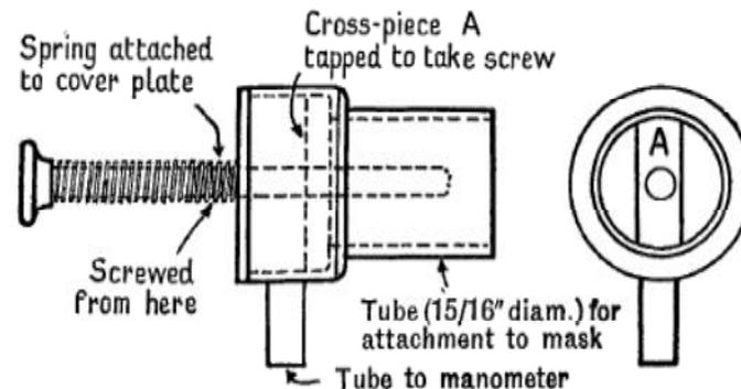
The pressure in the air passages is regulated by the strength of the spring and by the rate of flow, and the two should be adjusted so that there is an insignificant fall in pressure in the manometer during inspiration. A plus pressure of 6 in. is about the maximum that can be tolerated;
