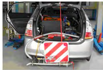
(ii) PEMS installation
