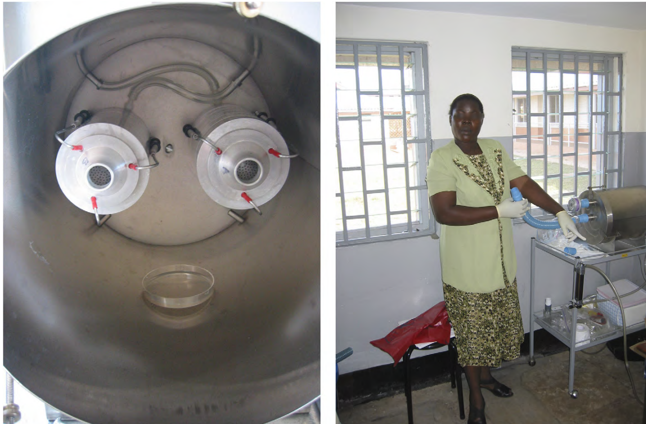
Figure 1. Cough Aerosol Sampling System. View inside of chamber with two Andersen cascade impactors and settle plate (left) and set up in procedure room ready for use (right).
